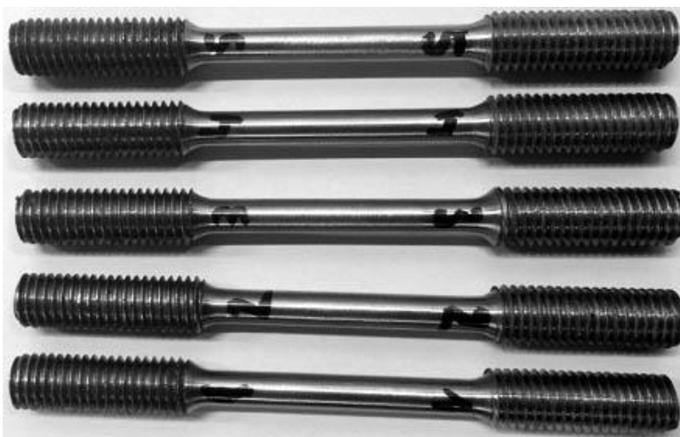
Figure 5. Specimens for static tensile test.
