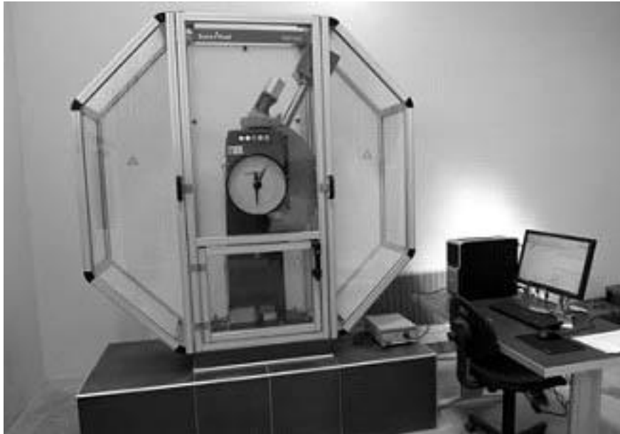
Figure 3. Instrumented Charpy testing machine RKP 450.
