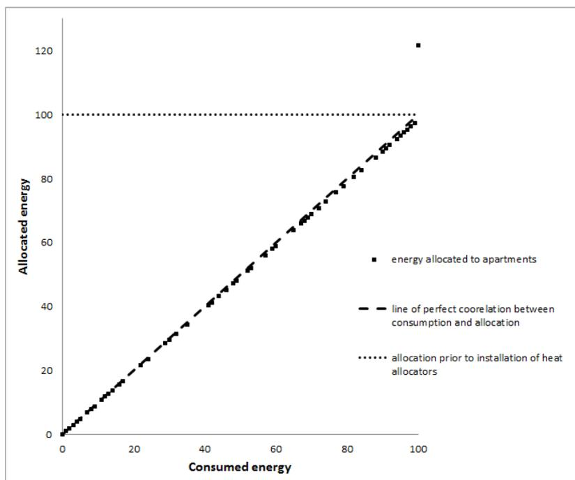
**Figure 8.** Comparison of energy allocation and energy consumption according to proposed formula.
