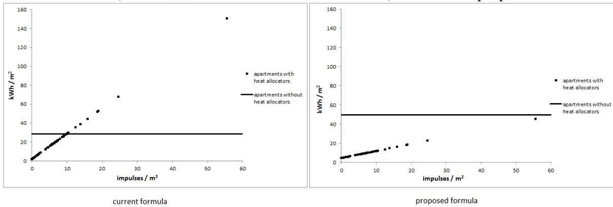
**Figure 13.** Comparison of allocated energies for an apartment building in city of Slavonski brod, based on measuring taken in December of 2012.
